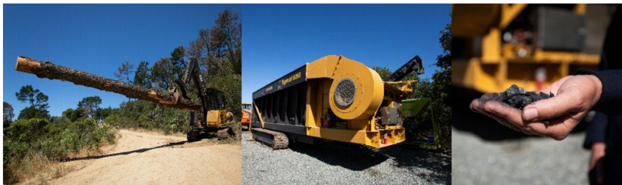
As part of fuels reduction work for fire suppression a tree is removed then burned in a low-emission Tigercat 6050 carbonator machine, resulting in biochar used to enrich soil in the East Bay parks. Photos: EBRPD
